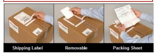
The shipping label is printed and held on the applicator tamp. The packing sheet is printed, folded and applied to the bottom of the shipping label. The shipping label is then applied to the top of the carton with the packing sheet securely placed under the removable label.
